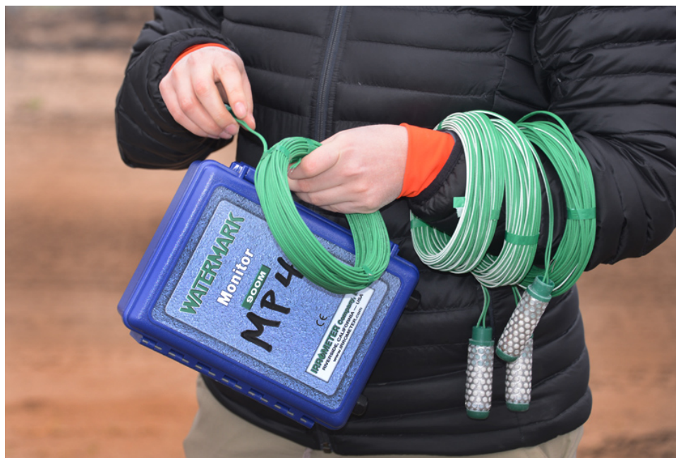
Installation of Watermark Sensors.
