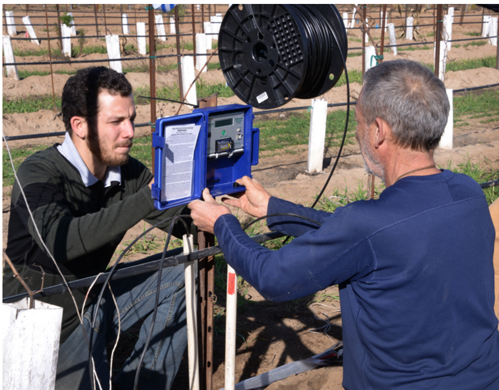
Installation of Watermark Sensors.
